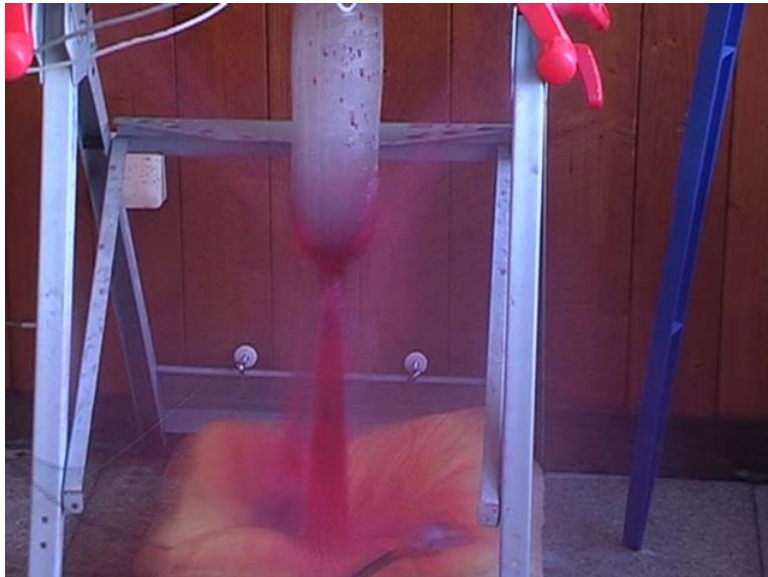
Fig. 7: Water expulsion at t = 0.01s
