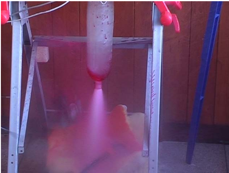
Fig. 9: Air-water expulsion with formation of a clockwise turning water vortex at t = 0.05 .
