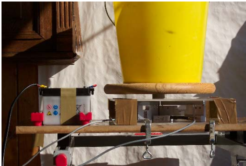
Fig. 3: Calibration with standard weights (liters of water in the bucket)
