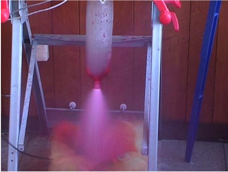
Fig. 8: Air-water expulsion at t = 0.02\text{s}
