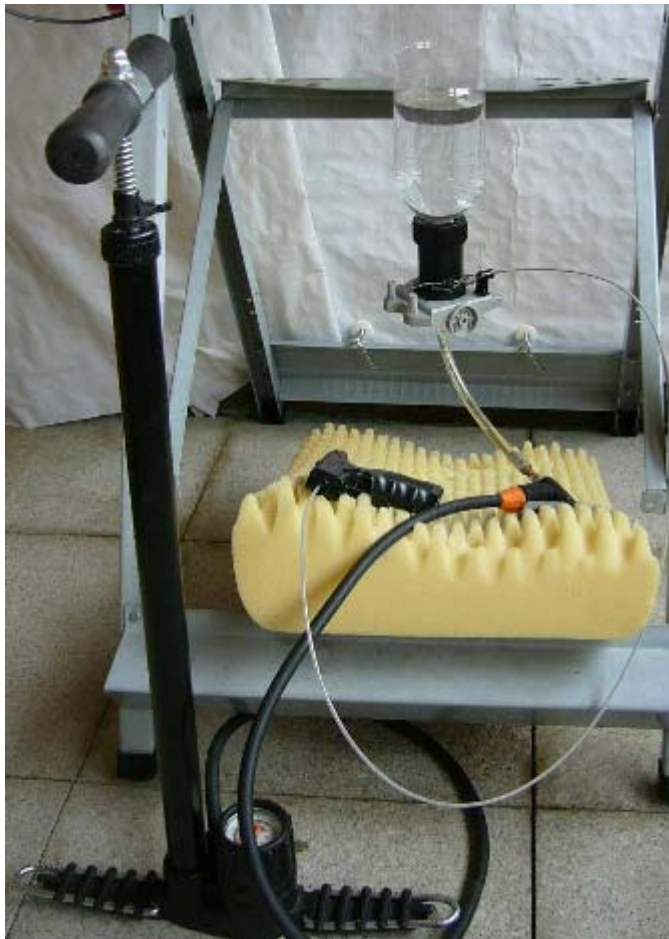
Fig. 5: Air pump with pressure gage and release mechanism with pistol trigger of a Shooter 9 water rocket. The yellow cushion serves as a damper.
